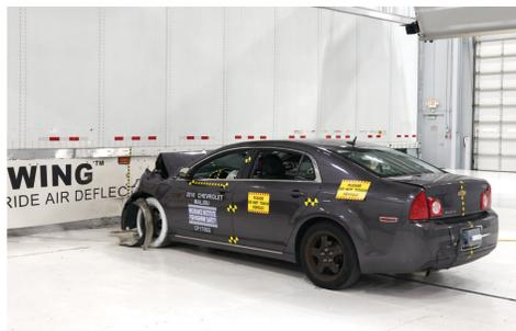
The Institute has been testing rear underride guards for several years. In March, IIHS announced the first winners of the new **TOUGHGUARD** award recognizing rear underride guards designed to prevent underride in a range of crashes into the backs of tractor-trailers. So far, five North American semitrailer manufacturers have qualified for the award.
